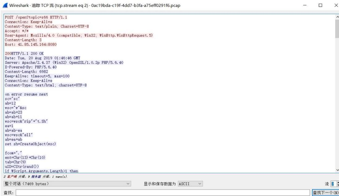
The role of this vbscript is to collect user host information (user name, host name, host installation configuration information, system version information, network card information, ip, etc.), system current process information, and then return this information to the C&C server. The C&C address is still the IP coded in the first vbs: 41.85.145.164: 8080
